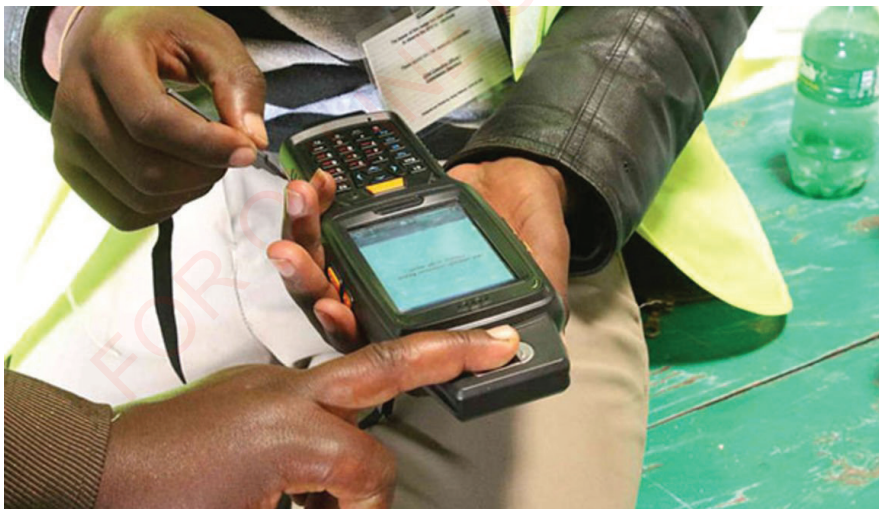
Figure 3.2(a): Fingerprint biometric device to secure identification
