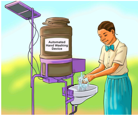
Figure 5.3: Solar powered automatic hand-washing device
