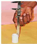
Figure 3.11: Measuring depth using the vernier caliper
