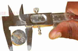
Figure 3.9: Measuring external diameter using the outside (lower) jaws
