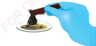
Figure 6.2: Magnetic separation of a mixture of sulphur and iron filings
